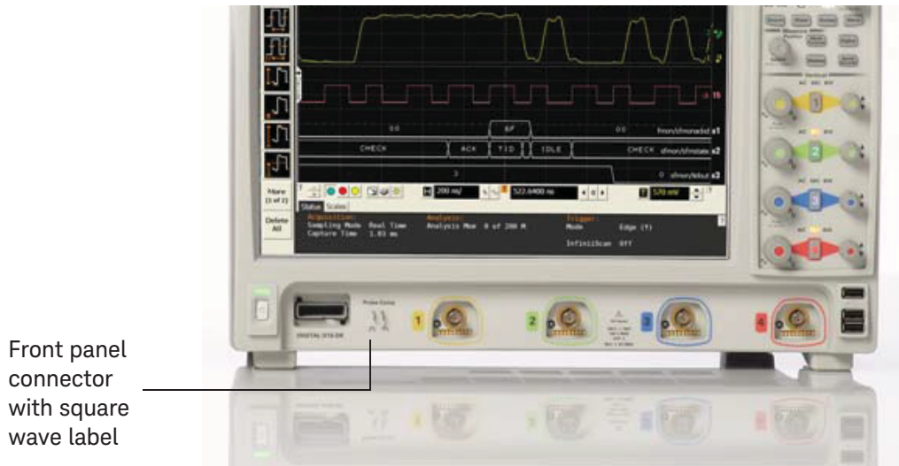
Figure 6 Verifying basic oscilloscope operation
