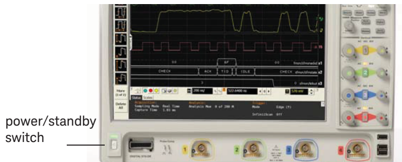
Figure 5 Turning On the oscilloscope
